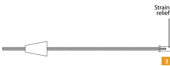
**3** Insert the coaxial cable through the flared end of the strain relief.
