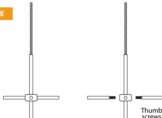
**2** Remove the three thumb screws.
