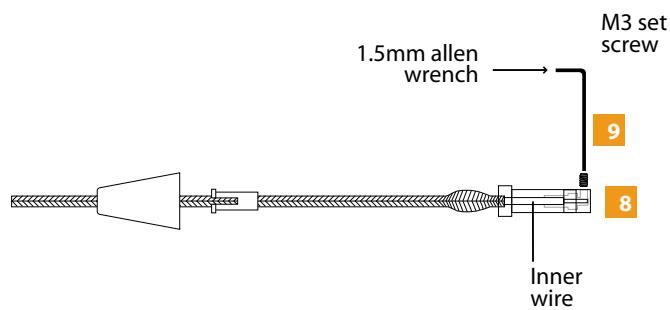
**8** While inserting the inner wire into the connector look through the set screw hole to make sure that the stripped portion of the inner wire contacts end of the connector.
