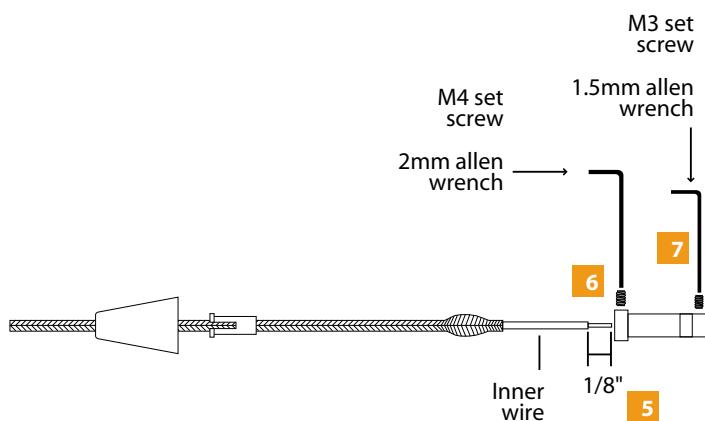
**5** Strip 1/8" from end of the inner wire. Make sure that the stripped portion is not greater than 3/16".
