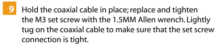
**9** Hold the coaxial cable in place; replace and tighten the M3 set screw with the 1.5MM Allen wrench. Lightly tug on the coaxial cable to make sure that the set screw connection is tight.
