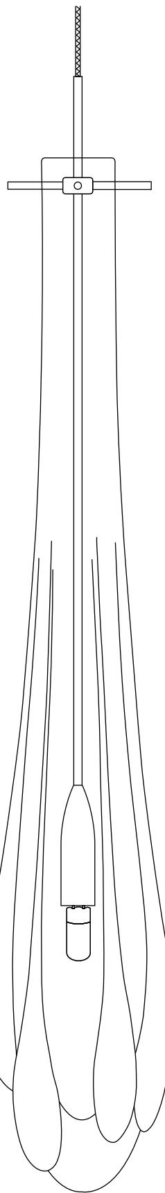
**3** Place the glass shade completely into the ring and tighten the three thumb screws to secure the glass shade in place.
